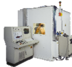
Robot based System for high throughput inspection of general castings
