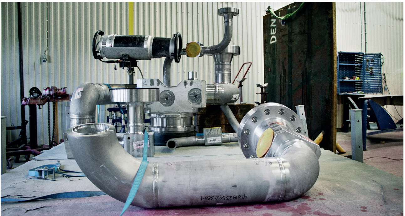
A Comet EVO 300DS positioned for inspection of pipeelements in one of the bunkers at the Verdal facilities
