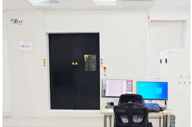
The HR 225C offline CT system, featuring Comet MesoFocus 225, will be delivered to at least 18 battery factories across regions in China.
