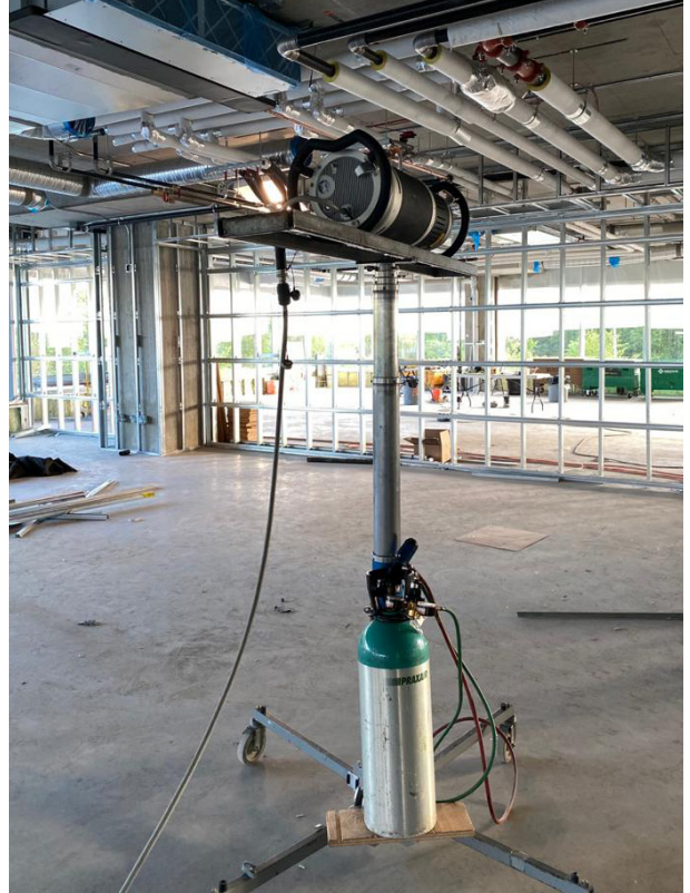
The Comet X-ray EVO 300D setup on SuperHoist - ready to shoot.
