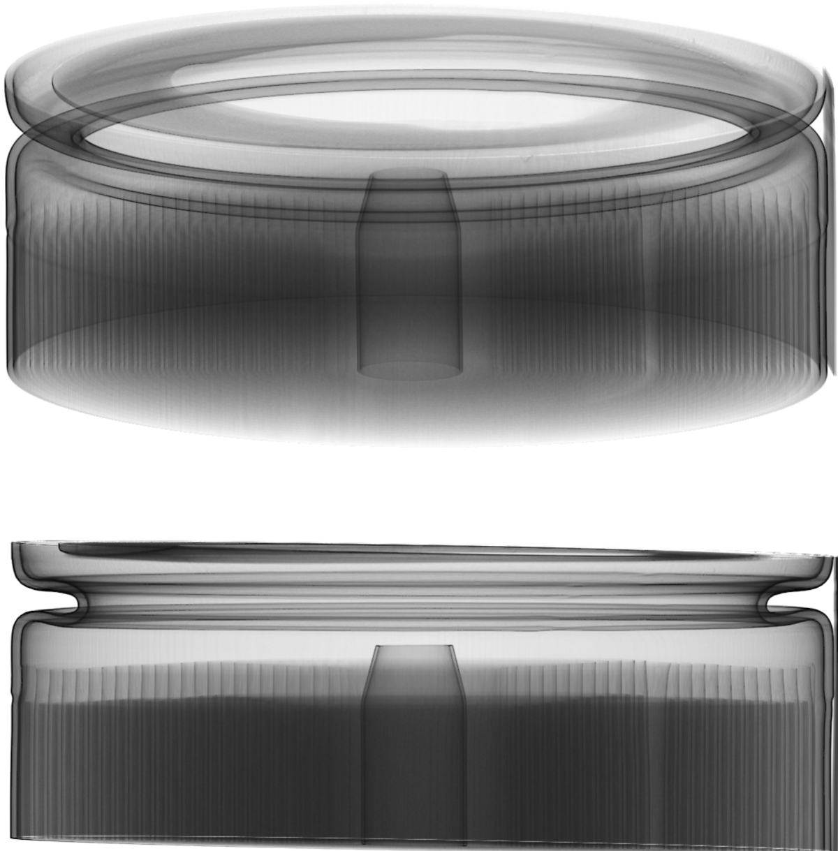
Figure 1: Angled and parallel views of a cylindrical battery cell in a 2D X-ray image
